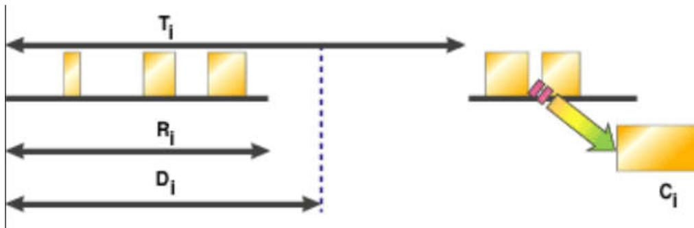
$$R_i = C_i + \sum_{\forall k \in hp_i} \left\lceil \frac{R_k}{T_k} \right\rceil C_k$$
