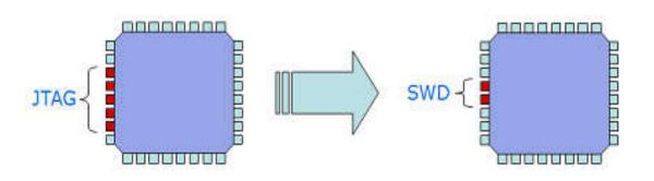
The Cortex CoreSight debug system uses a JTAG or serial wire interface. CoreSight provides run control and trace functions. It has the additional advantage that it can be kept running while the STM32 is in a low power mode. This is a big step on from standard JTAG debugging.
